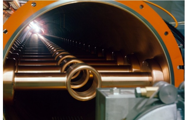
Fig. 5: Internal structure of the SPS travelling wave cavity
