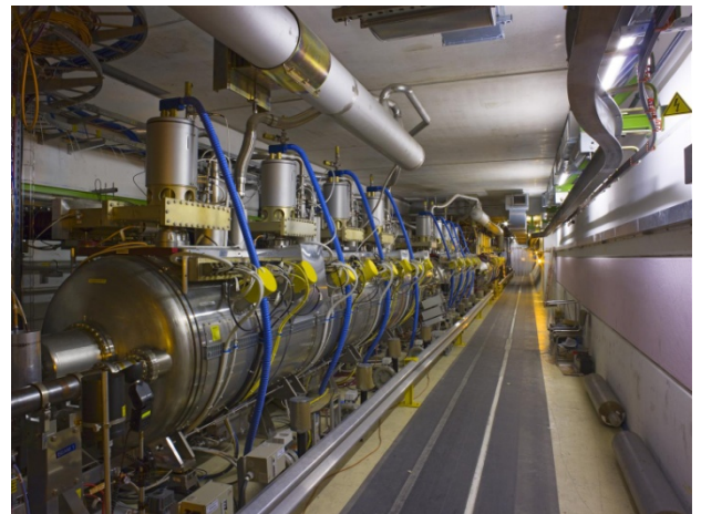
Fig. 9: Accelerating cavities at LHC Point 4. The cryomodule contains 4 cavities. The power coupler of each cavity with the waveguide feeder line is visible on top of the module [30].
